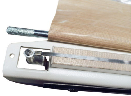
Figure 8. Remove heating element from mounting spring
