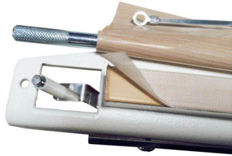
Figure 9. Remove PTFE adhesive
